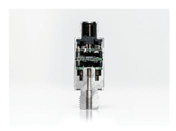
Cross section through a pressure transmitter. In the case of relative pressure transmitters, the inside space above the measuring membrane (on the side facing away from the medium being measured) must, under certain conditions, be connected to the environment in such a way that pressure equalization to the atmosphere can take place.
