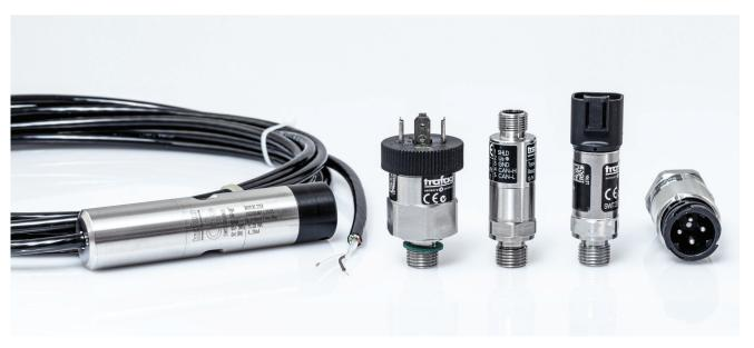
Comparison between various venting concepts for pressure transmitters. From left to right: vent tube in the cable (here with a level sensor); device plug to DIN 43650-A with low protection level; M12x1 plug with hole in protected thread area (gore membrane
